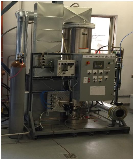
QuantumPure™ Automatic Cryogenic Purifier
